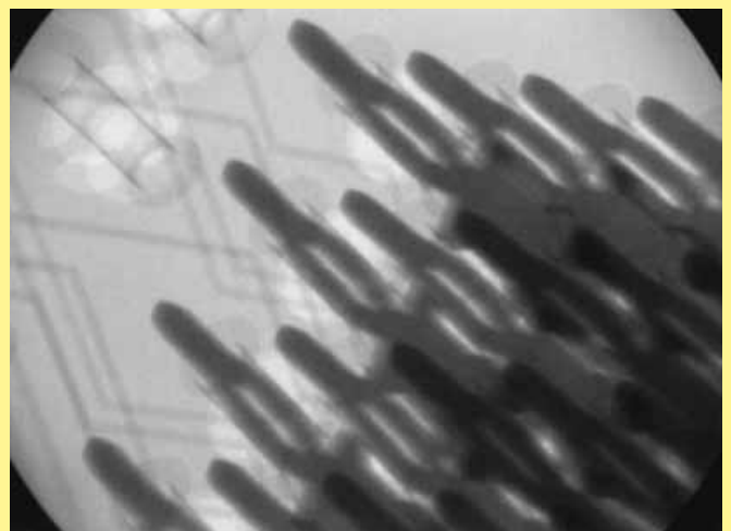
X-ray photo of a pressed-in connector
